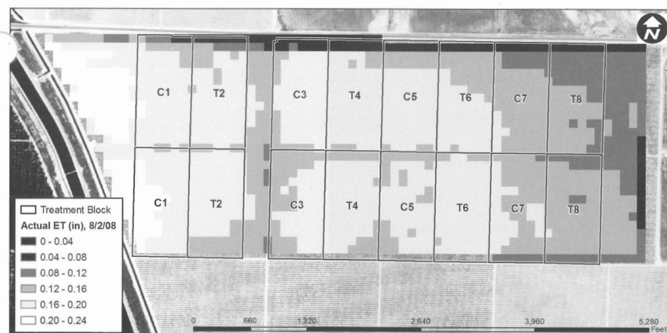
Figure 3. ET_a on August 2, 2008, for the ITRC study field. From the Surface Energy Balance Algorithm for Land (SEBAL ® ) and LandSat Imagery.
