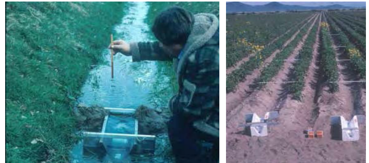
Figure 7. — Portable RBC Flumes Measure Flow in Drains and Furrows.
