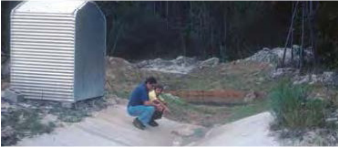
Figure 6. — Triangular-Throated Flume in Florida.
