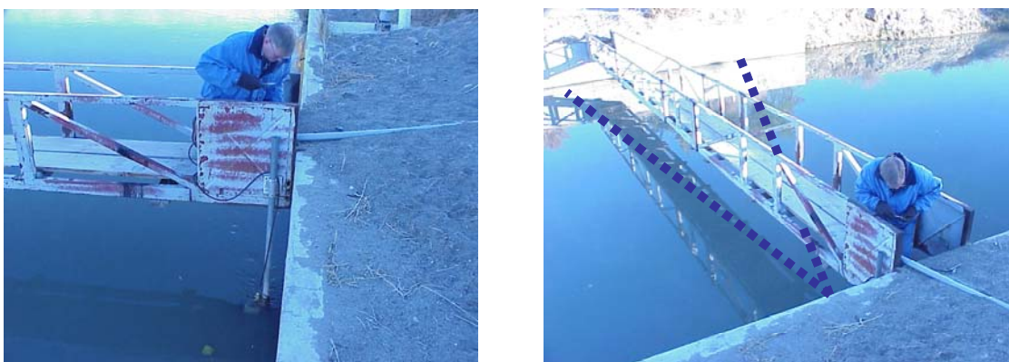
Figure 4. SonTek/YSI Argonaut SL installed in a canal
