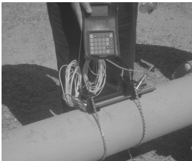
Figure 10. Portable ultrasonic flow meter on outlet pipe of an irrigation well. Sensors are usually mounted on the side of pipe to avoid air bubbles that may be in the pipe.
