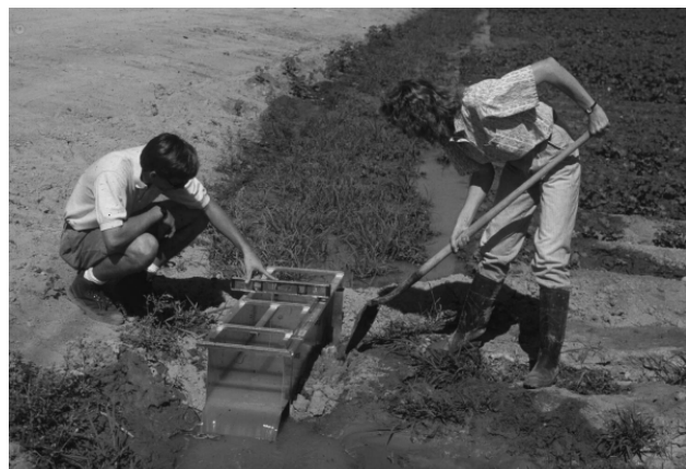
Figure 7. Adjustable flume being installed while channel continues to flow. Capacity: 56 L/s (2 cfs).
